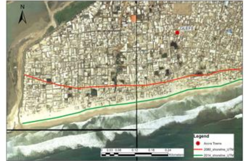
Glefe area eroding over 161 m from 2014 position
